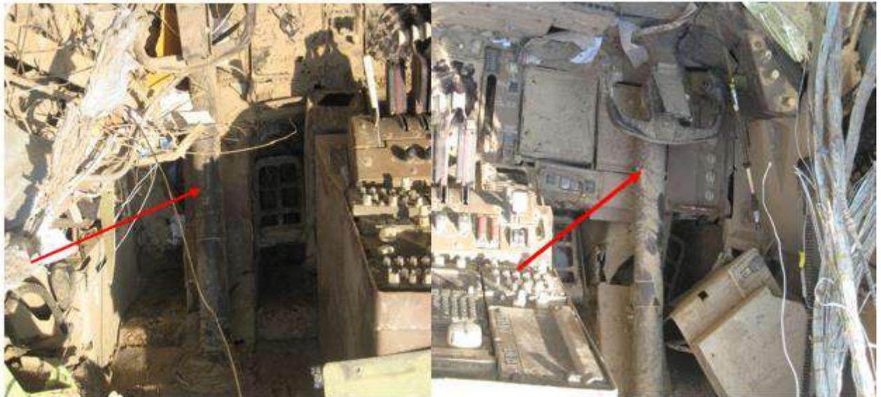
**Figure 10. Pilots' control columns (indicated by arrows)**
