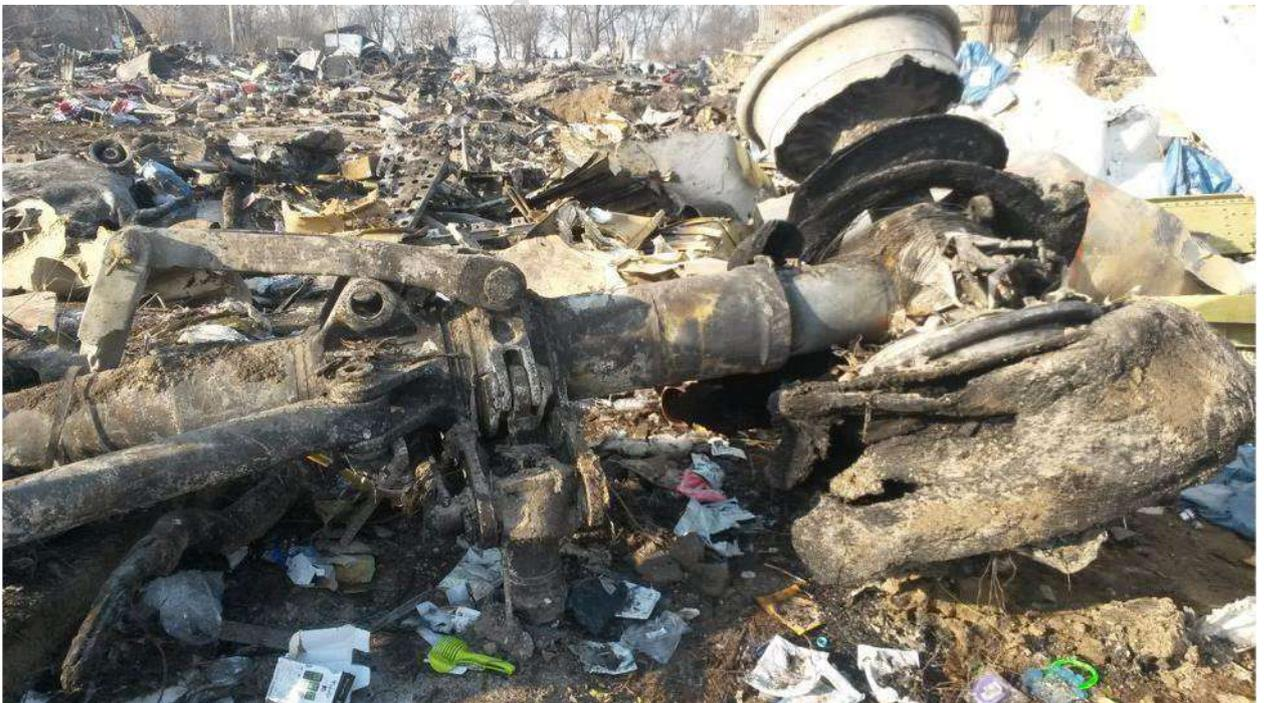
**Figure 6. Nose landing gear**
