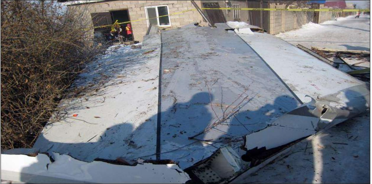
**Figure 29. RH wing tip with winglet**
