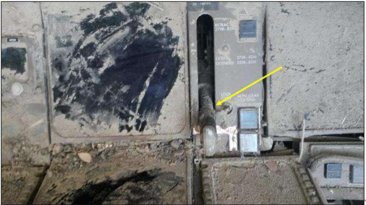
Figure 7. Landing gear extension/retraction control lever
