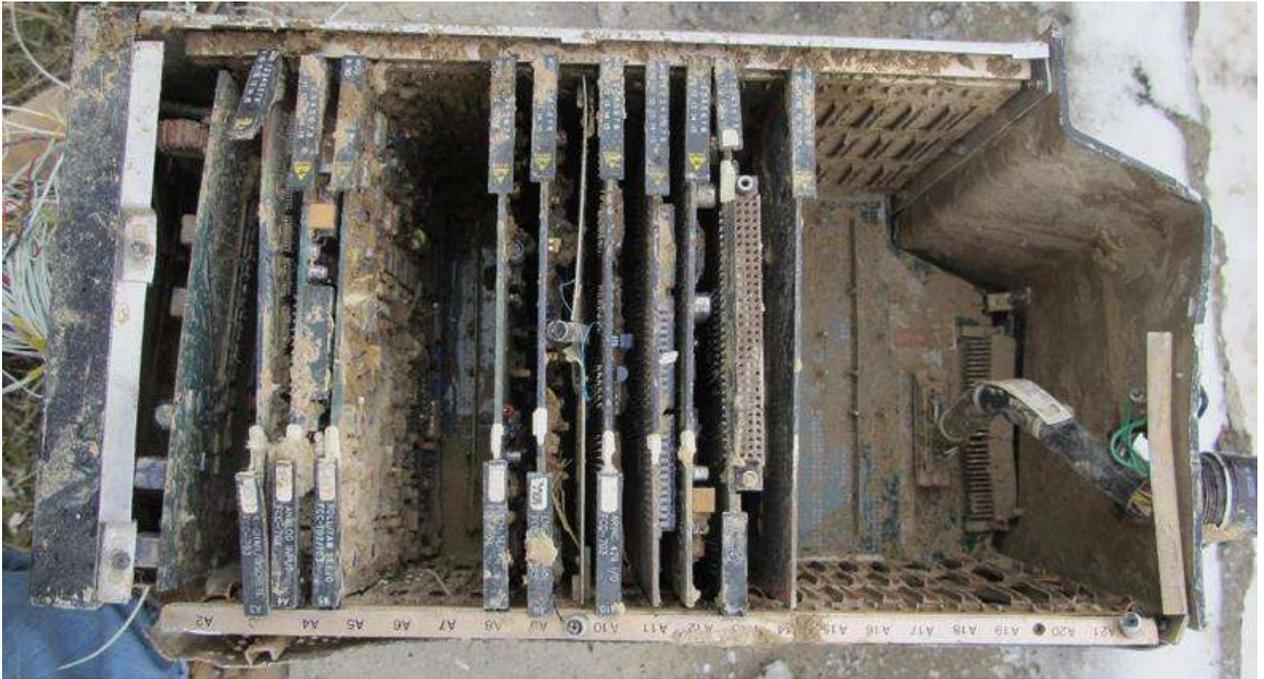
**Figure 11. FCC unit with remaining electronic circuit boards**
