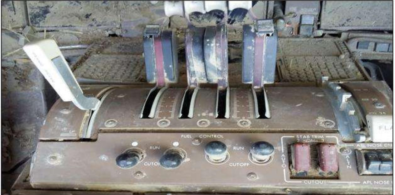
**Figure 9. Flap control lever**
