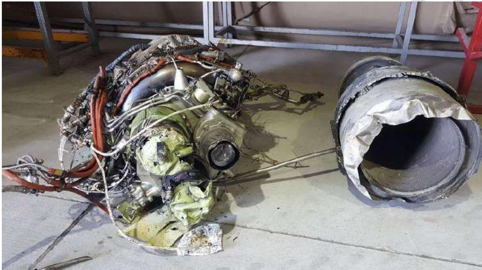
**Figure 17. Dismantled APU with APU exhaust nozzle**
