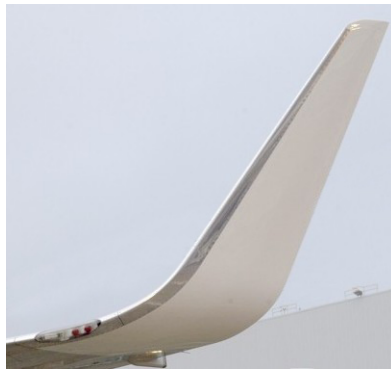
Figure 5.1. API blended winglet configuration for the 737NG family
